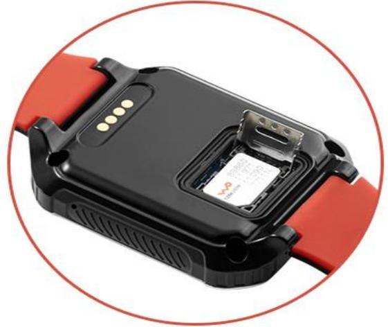
1. Unclench the lid of SIM card slot with tool 2. Insert the SIM card into the card slot
